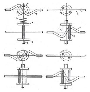
Fig.1 four Views of Simple Oscillating Mechanism
