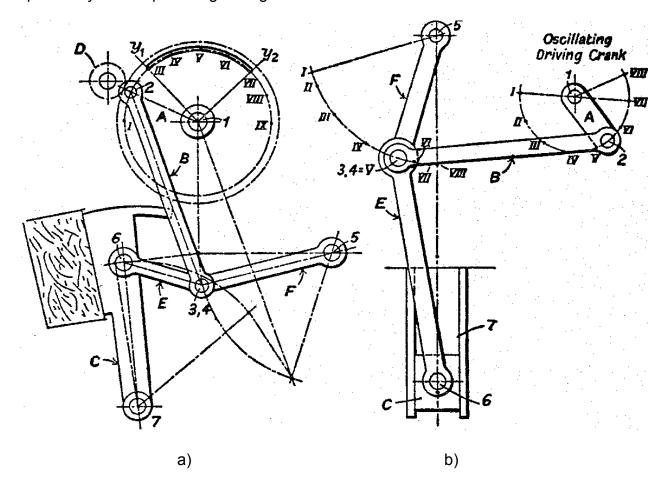
Fig. 3 Mechanism Double Toggle-lever for Straw-baling Press.
